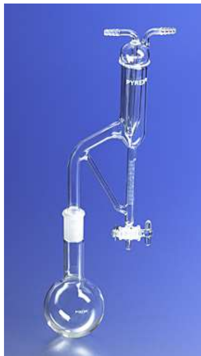
Clevenger Apparatus (Oil lighter than water)
