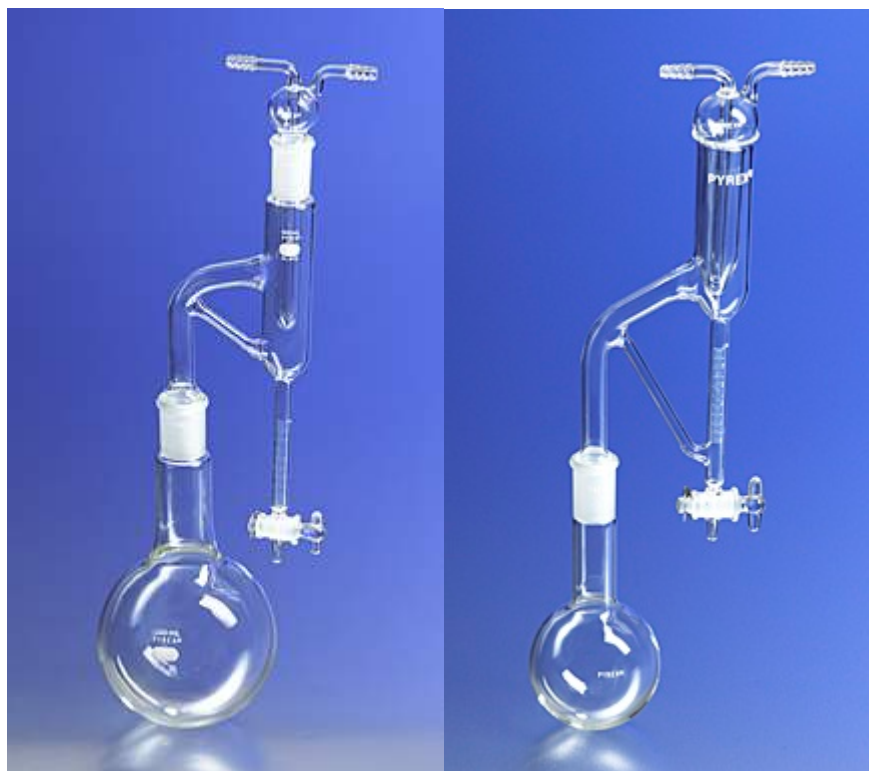
Clevenger Apparatus (Oil heavier than Water)
